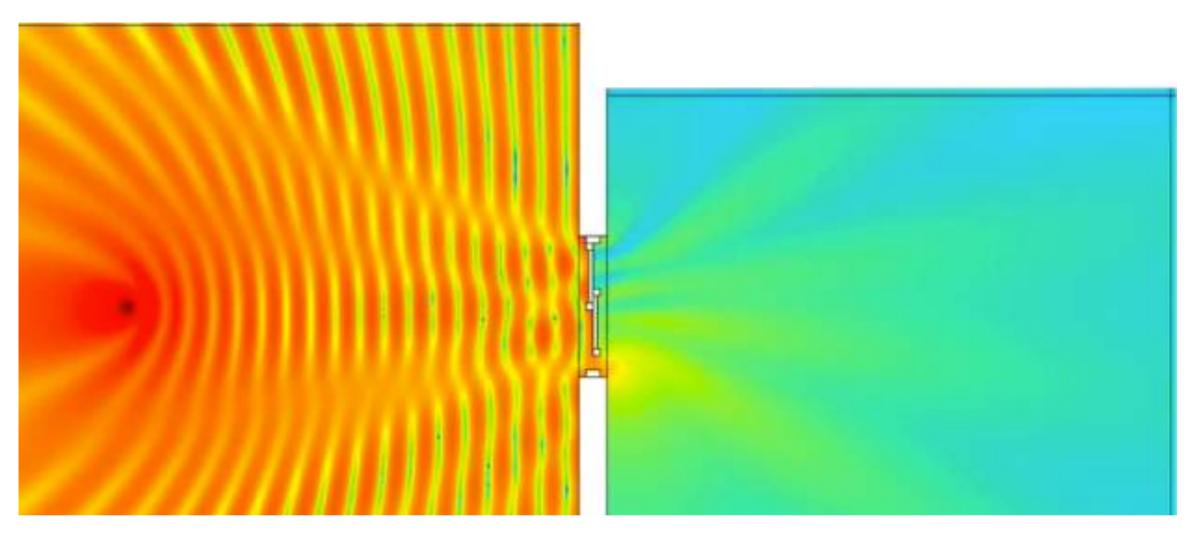
This video shows the impact of an internal baffle on sound reduction of an open window.
