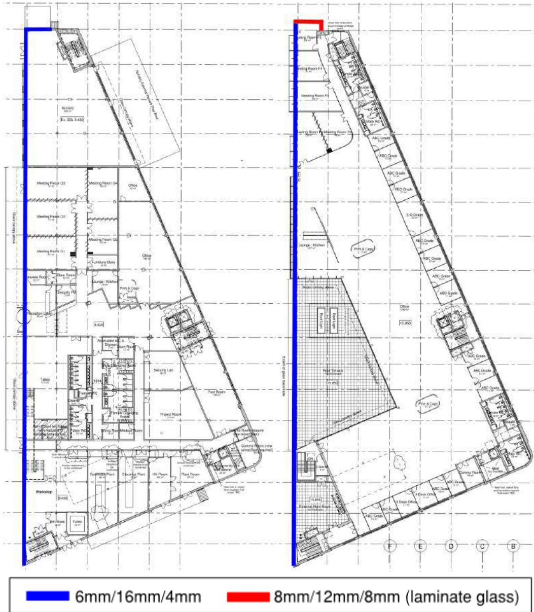
Figure 1: Façade glazing requirements for ground and first floor
